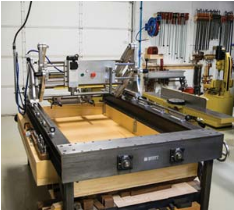
My single spindle gunstock duplicator. Capacity is 14” in diameter by 53” long.
